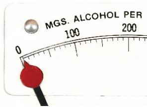
Figure 7. The Breathalyzer's BrAC scale. Note the start line to the left of the zero point. Subject tests began with the BAC pointer repositioned to the start line to negate or reduce the possibility of endogenous contamination affecting the reported BrAC results.
