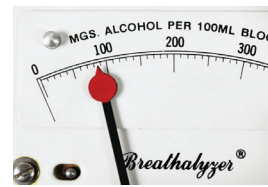
Figure 13. Increments on the BrAC scale were small, and their interpretation left to the judgement of the trained operator.
