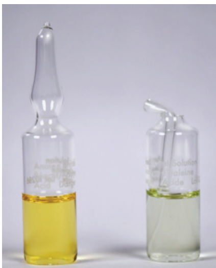
Figure 9. The reference ampoule, left, retains its original color while the test ampoule, right, has changed significantly.
