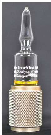
Figure 4. An ampoule in the “go” side of the go/no-go gauge.
