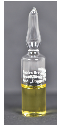
Figure 2. The proprietary ampoule of reagent solution designed and manufactured specifically for the Breathalyzer.
