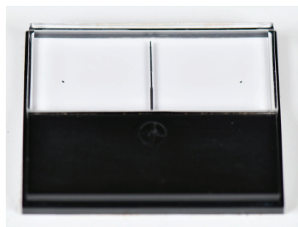
Figure 6. The Breathalyzer’s null meter, used to balance the optical array.
